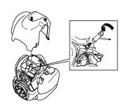
Clean, gap or replace the spark plug.
