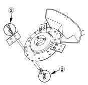
When replacing the blade, change the nuts and washers Saat penggantian pisau, ganti mur dan cincin penutup.
