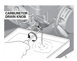
3. After all the fuel has drained into the container, tighten the drain knob securely.
