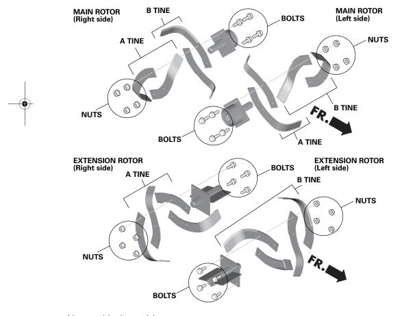
Nut and bolt positions For all rotary tines: Tighten the bolts from inside out.
