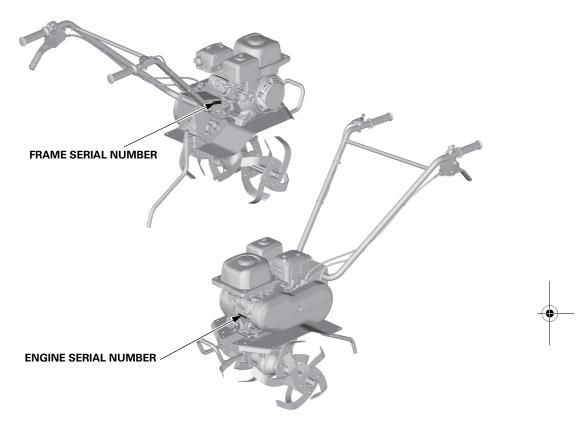
Record the engine and frame serial numbers in the spaces below. You will need these serial numbers when ordering parts, and when making technical or warranty inquiries.
