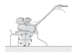
Remove the fuel tank cap and check the fuel level. Refill the tank if the fuel level is low.
