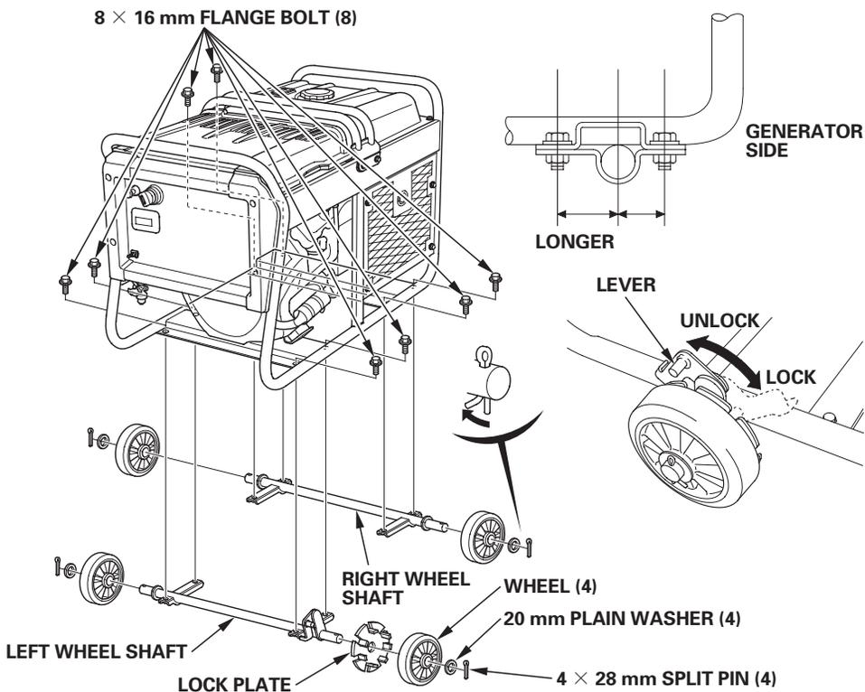
The wheels can be locked by turning the lever. Use the wheel lock when necessary.
