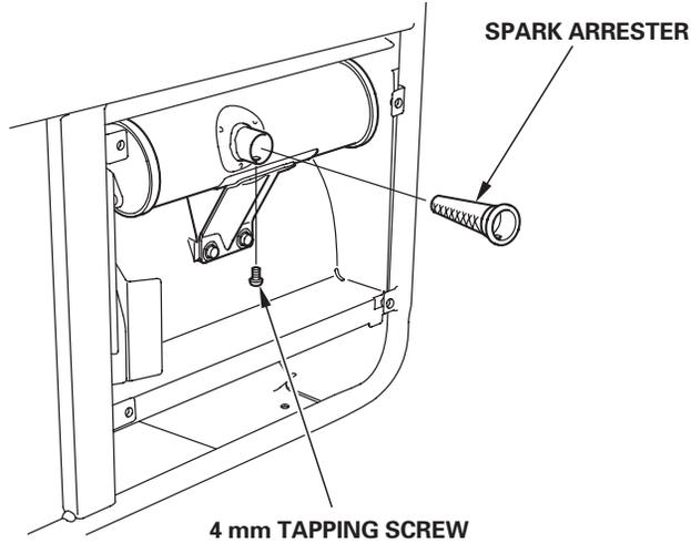
3. Use a brush to remove carbon deposits from the spark arrester screen.
