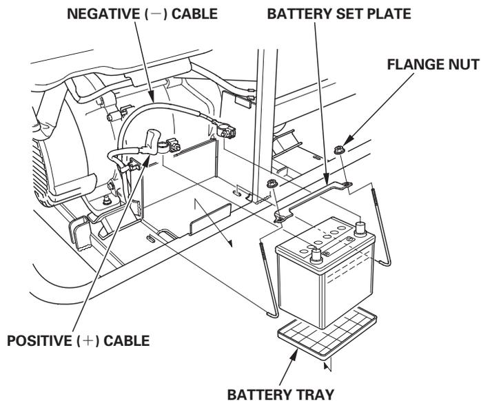
2. Remove the flange nuts, and remove the battery set plate.
