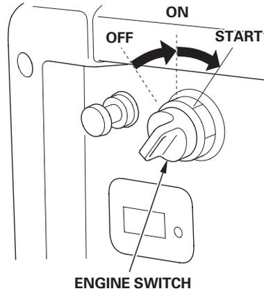
Do not leave the engine switch in the ON position when the generator is not operating as the battery will be drained. Turn the engine switch to the OFF position when not in use.
