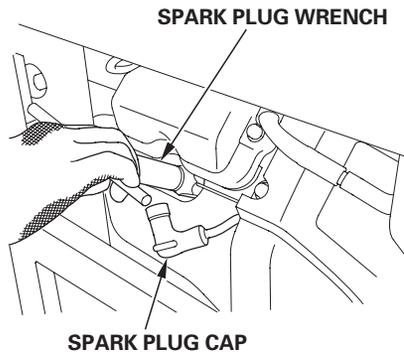
3. Inspect the spark plugs. Replace them if the electrodes are worn or if the insulator is cracked, chipped, or fouled.
