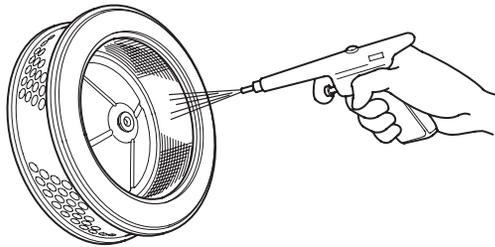
Never try to brush off dirt; brushing will force dirt into the fibers. Replace the paper filter element if it is excessively dirty.
