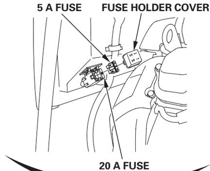
2. Remove the fuse holder cover and pull the fuse out.
