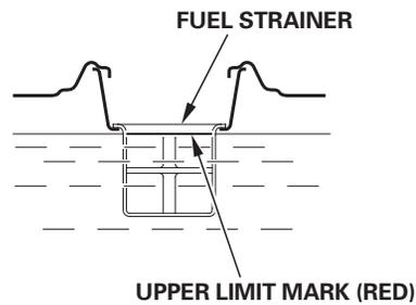
Refuel in a well ventilated area before starting the engine. If the engine has been running, allow it to cool. Refuel carefully to avoid spilling fuel. Do not fill the fuel tank above the upper limit mark (red) on the fuel strainer.
