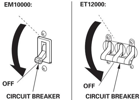
2. Turn the engine switch to the OFF position.
