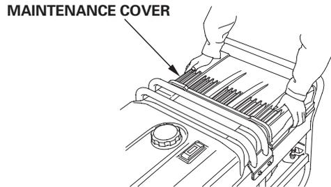
2. Pull the air cleaner cover latch to the unlocked position, and remove the cover.
