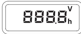
After showing all segments, the i-Monitor shows current accumulated hours and the battery voltage alternately for three seconds.
