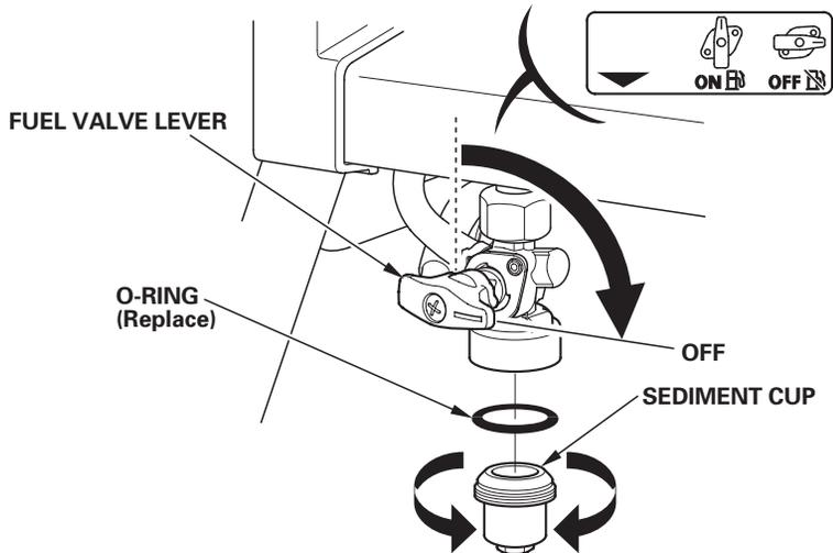
2. Clean the sediment cup in nonflammable solvent, and dry it thoroughly.
